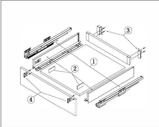
1. Guide Left/Right Length: 270mm, 300mm, 350mm, 400mm, 450mm, 500mm, 550mm
