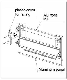
5. Install the assembled inner drawer front with the drawer sides
