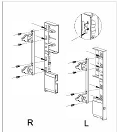
3. Connect the inner drawer front connector, front panel and front rail
