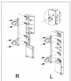
3. Connect the inner drawer front connectors, front panel and front rail
