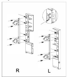
3. Connect the inner drawer front connector, front panel and square rail
