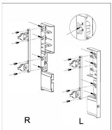
3. Connect the inner drawer front connector, front panel and glass front
